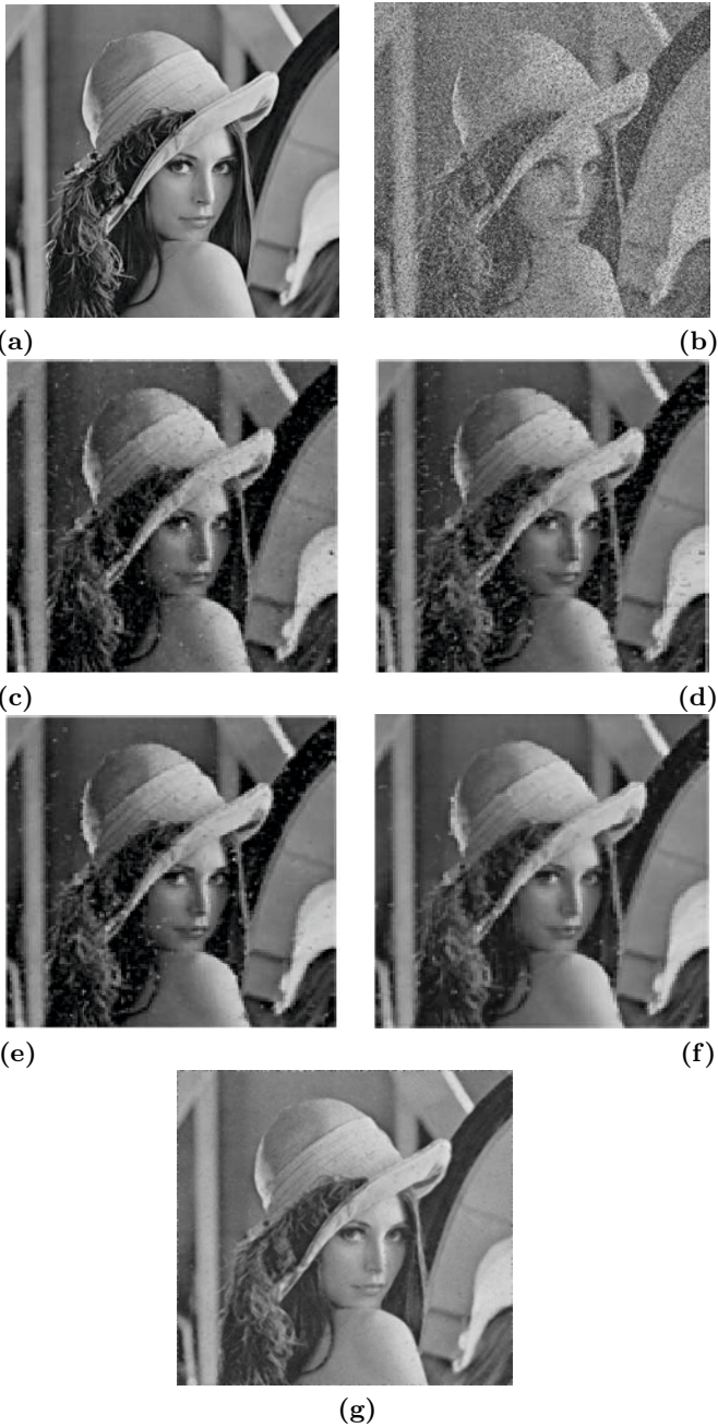
Fig. 2. Results of different filters in restoring 60% corrupted image Lena, (a) Original image (b)Noisy Image (c) (SD-ROM) [1] (d)(MSM) [5] (e)(PWMAD) [6] (f)(DWM) [8] (g)GADI(Proposed)
