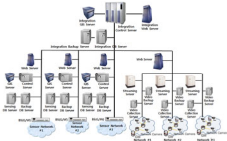
Fig. 6. Hardware Architecture for Sensor Networks and Video Networks
