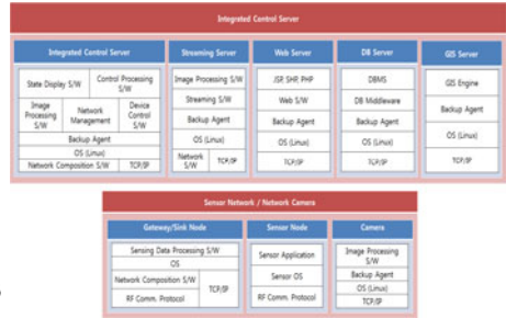
Fig. 7. Software Architecture for Sensor Networks and Video Networks
