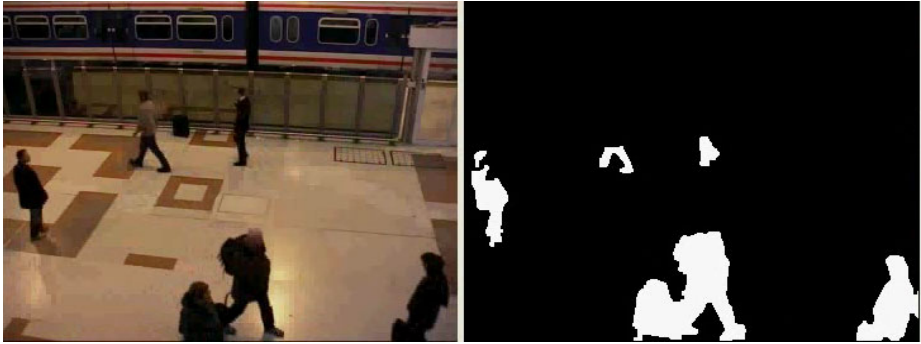
Fig. 4. (left) Six persons are moving, and two persons are close together. (right) Five blocks in addition to one large block.
