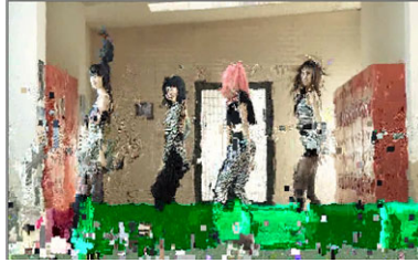
(c) Video frame sample with packet loss due to weak RSSI of WLAN
