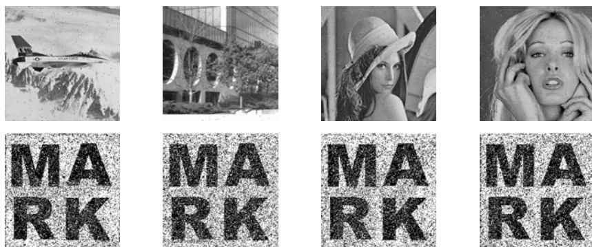
Fig. 8. Watermarked images with added salt & pepper noise (noise density: 0.005) and extracted watermarks
