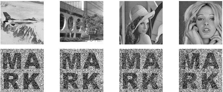
Fig. 7. Watermarked images with added Gaussian white noise (mean: 0; variance: 0.0005) and extracted watermarks
