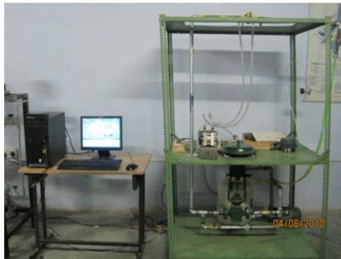
Fig. 1. Shows photograph of the pneumatic actuator system interfaced with PC using DAQ
