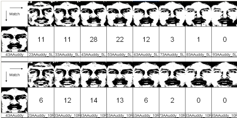
Fig. 10. Number of matched points between the frontal and posed faces with varying mask
