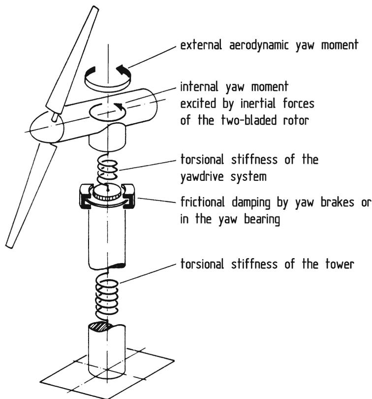
**Fig. 7.17.** Model of the vibrational behaviour of the yaw system
