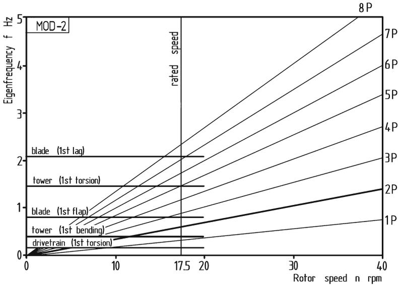
**Fig. 7.22.** Resonance diagram of the MOD-2 with teetering rotor on the upwind side and steel tube tower of soft design
