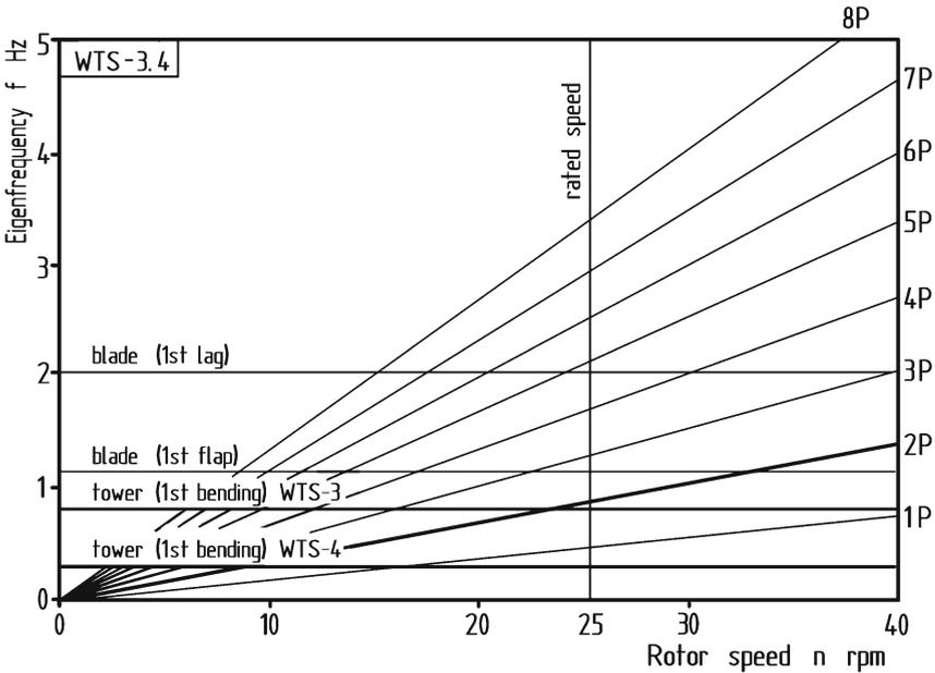
Fig. 7.24. Resonance diagram of the WTS-3/4 with two-bladed teetering rotor on the downwind side and soft tower design (WTS-3) as well as double-soft tower design (WTS-4)
