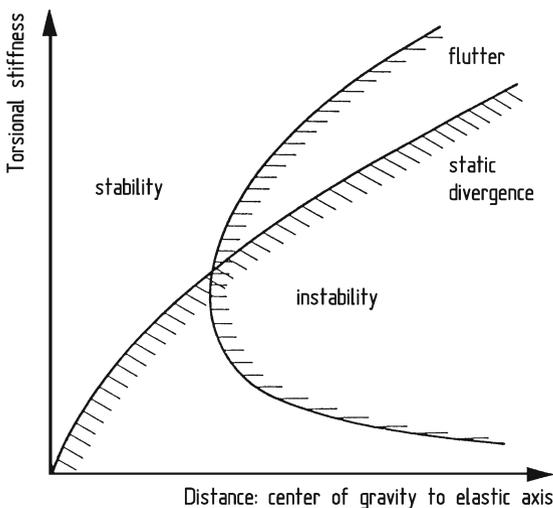
**Fig. 7.6.** Stability limits for the "static divergence" and "flutter" of wings and rotor blades [2]
