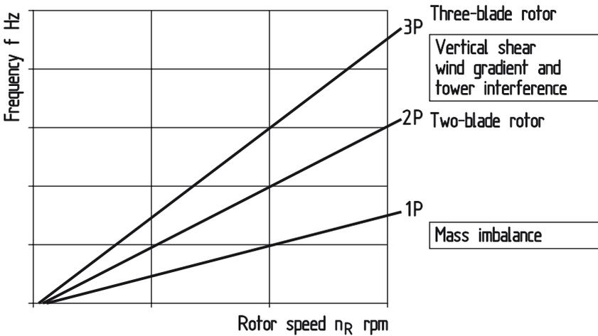
Fig. 7.2. Exciting frequencies as a function of rotor speed
