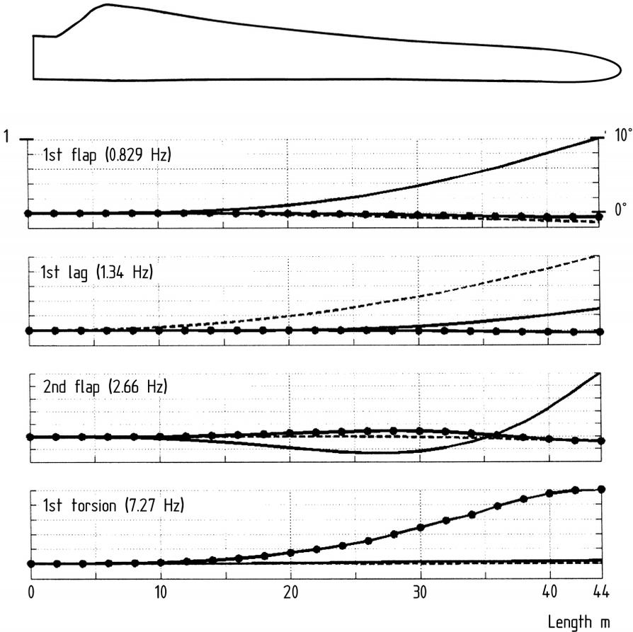
**Fig. 7.4.** Natural frequencies and eigenmodes of an Euro rotor blade of 44 m length [3]
