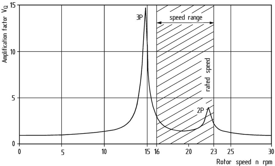
Fig. 7.27. Amplification of cyclic transverse force acting on the tower of the WKA-60 in a case of resonance
