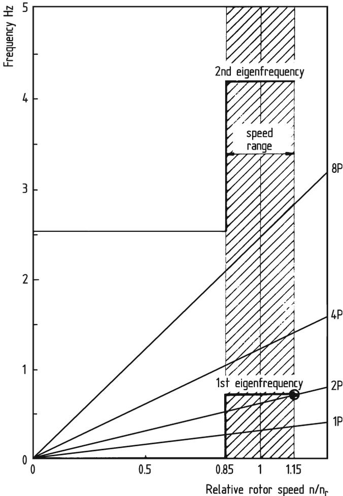
**Fig. 7.16.** Resonance diagram for the Growian drive train. Resonance of the first natural drive train frequency with tower shadow interference (2 P) at a rotor overspeed of 115 %
