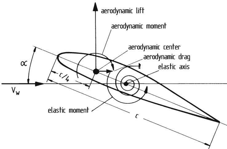
Fig. 7.3. Aerodynamic and elastic moments in a wing or rotor blade cross-section
