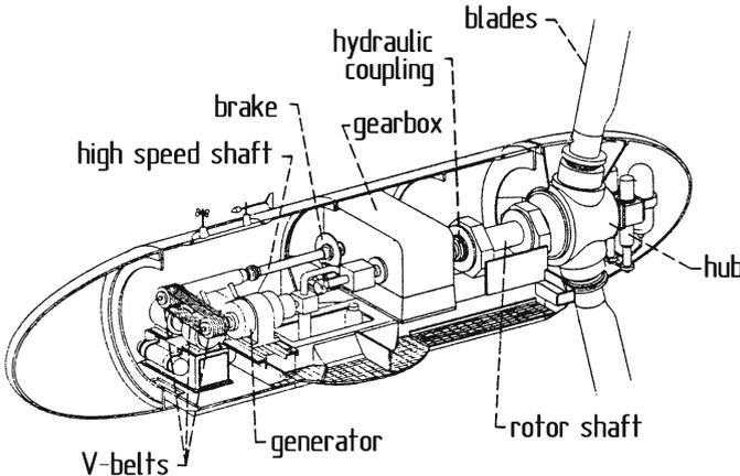
Fig. 7.13. Drive train of the experimental MOD-0 [5]
