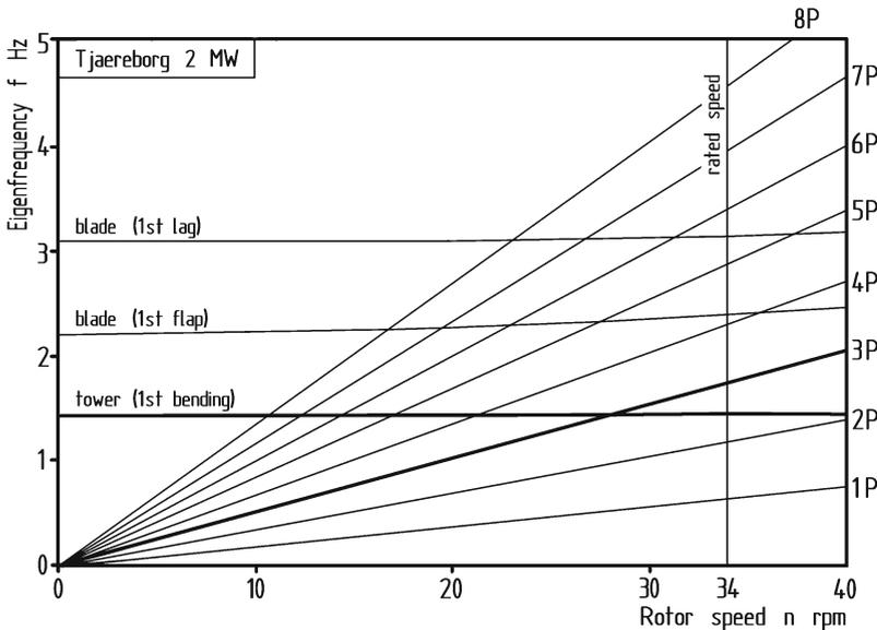
**Fig. 7.25.** Resonance diagram of the Tjaereborg turbine with three-bladed rotor on the upwind side and soft concrete tower
