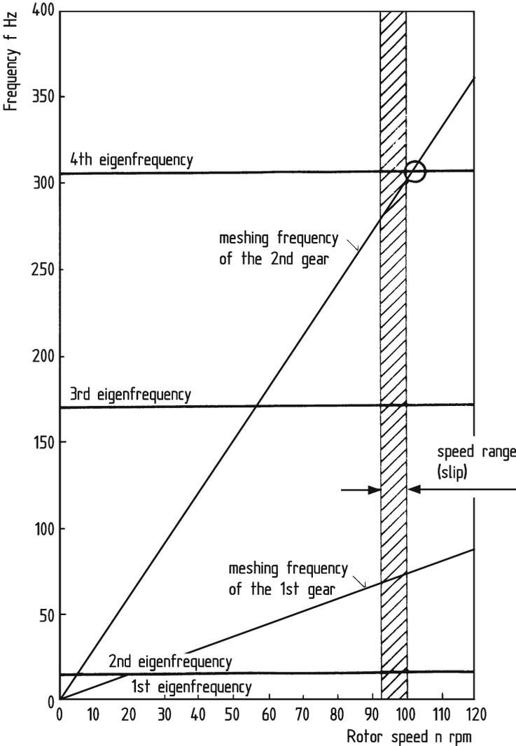
**Fig. 7.15.** Resonance diagram (Campbell diagram) of the Aeroman drive train with a resonant point at the fourth natural harmonic of the drive train, caused by the meshing frequency of the second gear stage close to rated operational speed
