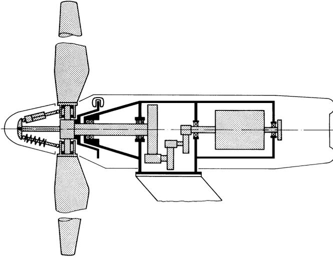
**Fig. 7.9.** Idealised drive train of a small turbine of the Aeroman type
