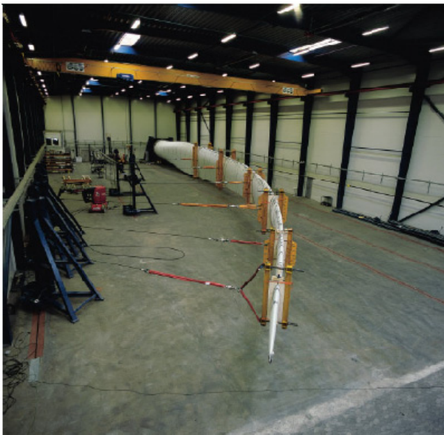
Fig. 6.36. Rotor blade test stand at LM Glasfiber
