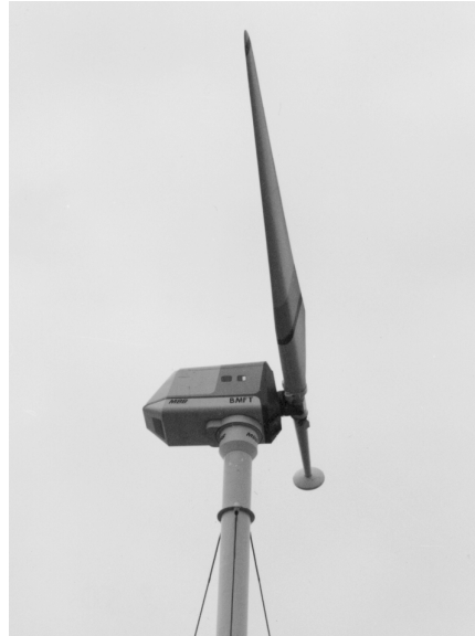
Fig. 2.28. Monopteros (rotor diameter 48 m, 600 kW), MBB (Germany), 1985
