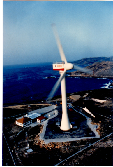
Fig. 2.39. Spanish AWEC-60 in the test field in Cabo Villano/North-Western Spain (rotor diameter 60 m, 1500 kW rated power), Union Fenosa, 1989
