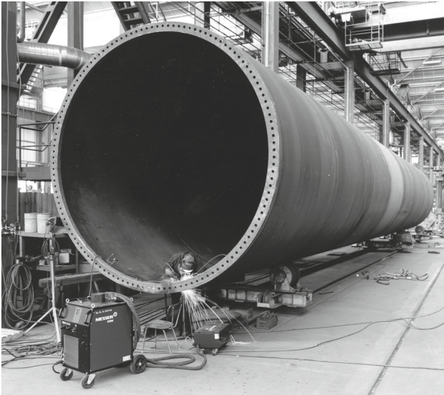
Fig. 12.12. Welding-on of the flange (CAS)
