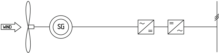
Fig. 10.34. Directly rotor-driven variable-speed synchronous generator with inverter
