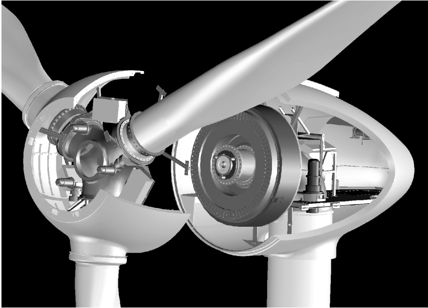
Fig. 10.35. Direct-drive multi-pole synchronous generator of the Enercon E-30
