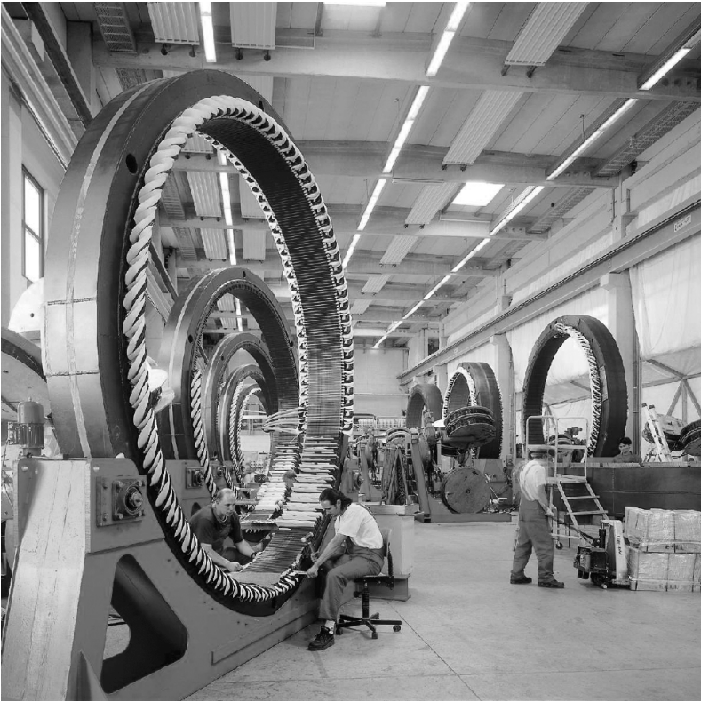
Fig. 10.36. Production of synchronous multi-pole generators by Enercon (Enercon)
