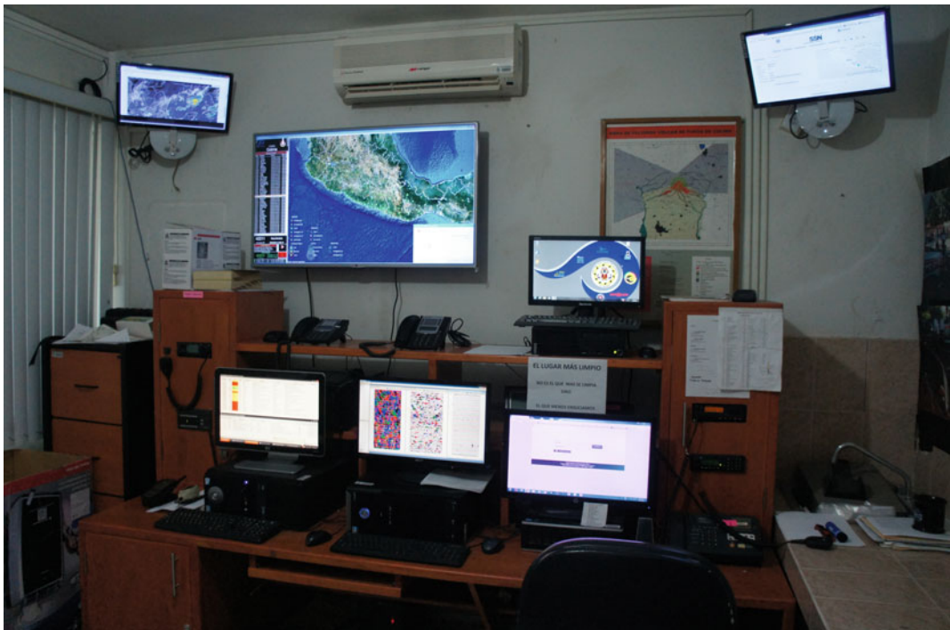
Fig. 4 State unit for Civil Protection’s communication centre. Real time seismic volcanic data can be observed on the lower and central screens. In theory, this centre functions as a monitoring and communication station for natural phenomena and the associated risk that occurs in
