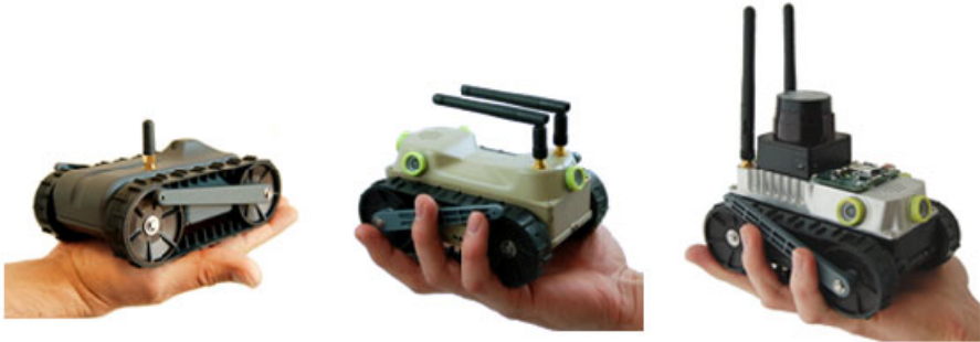
Fig. 2. Ember, the Phase I LANdroid prototype robot developed by iRobot (left), the Phase II LANdroid Development robot (LDR) developed by iRobot – standard top (middle) and sensor development payload bay top (right)
