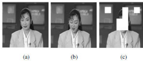
Fig. 2. The Sample output obtained from the motion estimation process in an akiyo video a) I-frame b) P-frame c) estimated motion in P-frame
