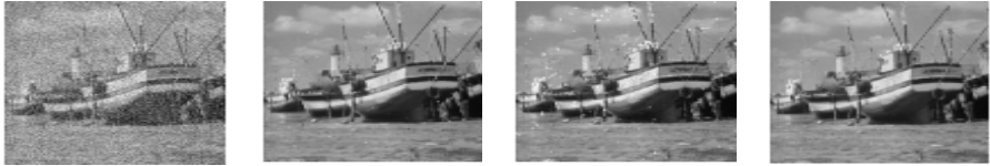
Fig. 2. Boat image corrupted by the Noise Model 2 with 25%, noise, Images restored by SODDWM, DWM and EWM filter respectively
