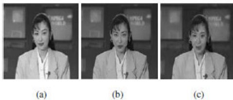
Fig. 3. The sample output obtained from the decompression process in an akiyo video a) Original frame b) Decompressed frame by proposed method c) Decompressed frame by FCWS video compression scheme
