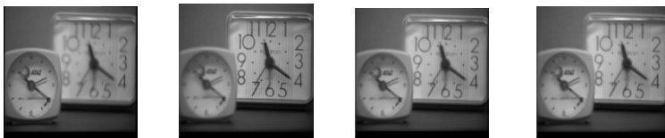
Fig. 6, 7, 8, 9. Left focused & Right focused source clock images, fusion output images for M = 1 and 2
