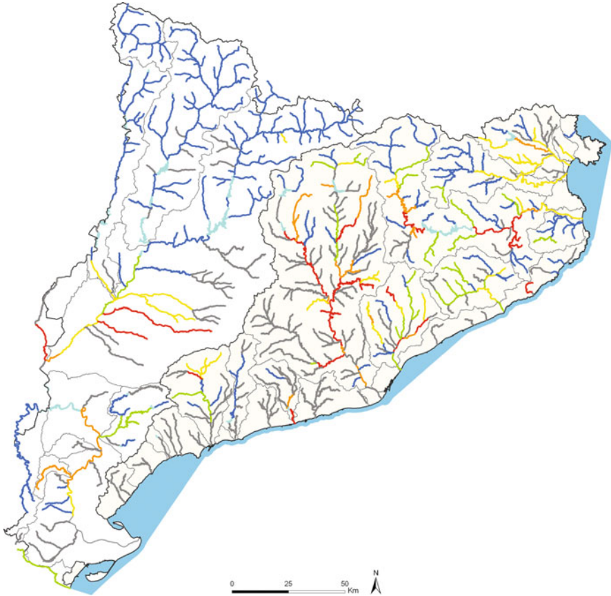
Fig. 4 Biological quality results using fish fauna (IBICAT index) in Catalan rivers (2007–2009). High quality is shown in blue , good quality in green , moderate quality in yellow , poor quality in orange , and bad quality in red color. Water bodies without data are shown in gray color. Reservoirs are shown in light blue
