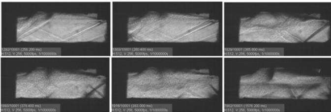
**Fig. 3** Schlieren pictures at different moments (from optical window 2).
