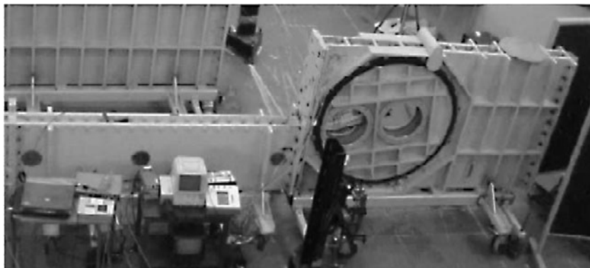
Fig. 1 Experimental layout showing the 1.1 m high test section with rotatable window frame connected to the 450 mm high shock tube driven section
