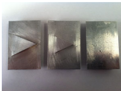
Fig. 1 Micro-ramp models of different sizes. MR-1 (left), MR-2 (middle) and baseline model (right).
