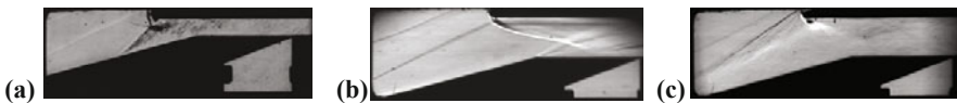
Fig. 4 Leading edge bluntness effect on the inlet starting characteristics. Cowl lip and forebody leading edge radius are r c , r f , respectively. Throat height h t . (a) h t =10mm, (b) and (c) r c =2mm, h t =20mm. (a)Run 309 un-starting inlet with r c =2mm blunted; (b)Run 355 self-starting inlet; (c)Run 366 unself-starting inlet with r f =3mm blunted.
