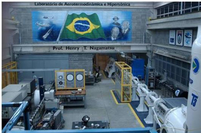
Fig. 1 Prof. Henry T. Nagamatsu Laboratory of Aerothermodynamics and Hypersonics. T2 Hypersonic Shock Tunnel, visible at the left of the T3 Hypersonic Shock Tunnel.
