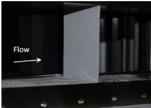
Fig. 3 Photo of the particle curtain acquired with a test section wall removed
