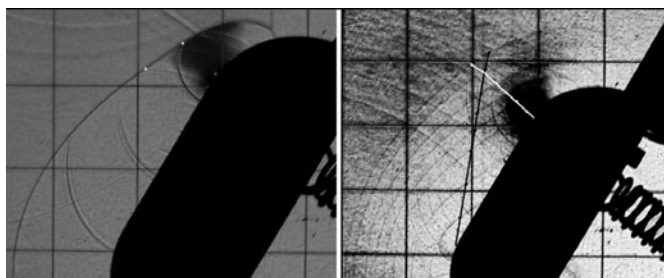
Fig. 5 Determination of the trajectories of how information from the changes in slope reach the reflected wave. The right image overlays a number of tests. The black line is for the P wave and the white line for the Q wave. The reflected wave remains plane between these lines until they meet
