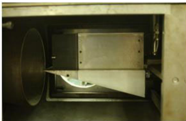
Fig. 3 Ramp Scramjet model used for supersonic combustion experiments.
