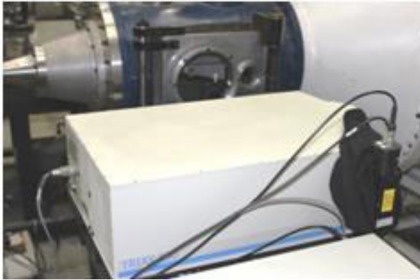
Fig. 4 Photography of experimental setup for time-resolved OH* emission measurements.
