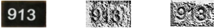
Fig. 3. The LBP feature images of different operator (the original image, the basic LBP operator, and the uniform pattern)
