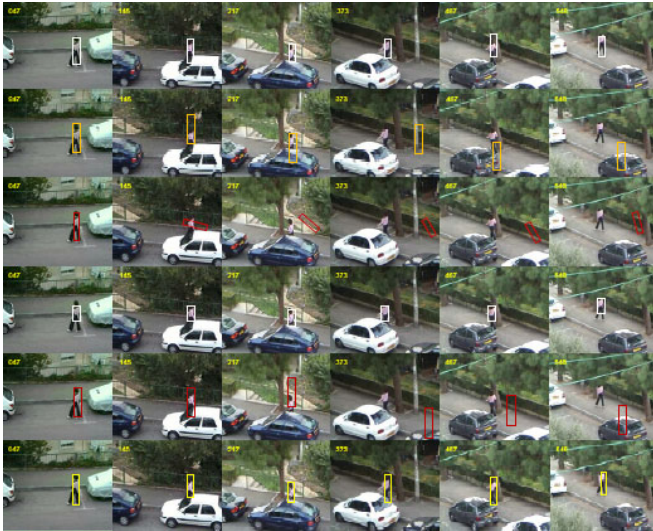
Fig. 4. Tracking results of the Walking woman sequence. From top to bottom are the results of IVT [13], MIL [2], GPF [9], GMS [14], Cov [12] and our method, respectively.
