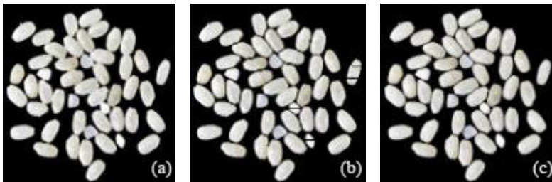
Fig. 3. Color image example and the segmentation results by MW and MSD; (a)color image example of rough rice; (b)segmentation result by MW; (c)segmentation result by MSD
