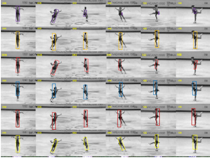
Fig. 2. Tracking results of the Female skater sequence. From top to bottom are the results of IVT [13], MIL [2], GPF [9], GMS [14], Cov [12] and our method, respectively.
