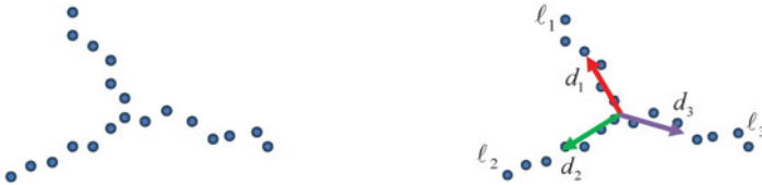
Fig. 2. Point cloud sparse decomposition. For a simple 2D example, n has been set to 3. Learned D has been shown as d_1, d_2, d_3 . Direction vector using the points in \ell_i decompose on D will only has a non-zero coefficient on d_i .
