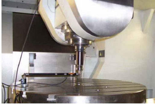
Fig. 5. DBB setup for rotary joint errors
