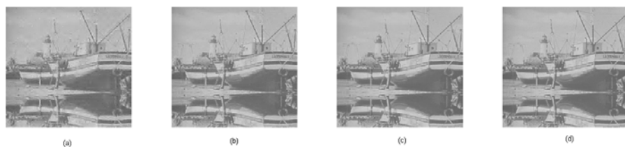
Fig. 3. The reconstruction results of Boat512 by FSAMP at different sampling rate (a) M/N=0.2 ; (b) M/N=0.4 ; (c) M/N=0.6 ; (d) original image
