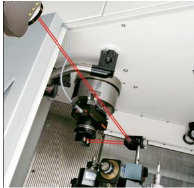
Fig. 4. Renishaw RX-10 setup for vertical axis roll errors
