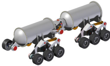
Fig. 1. Structure of composite wheeled submarine walking mechanism
