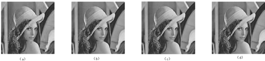
Fig. 2. The reconstruction results of Lena512 by FSAMP at different sampling rate (a) M/N=0.2; (b) M/N=0.4; (c) M/N=0.6; (d)original image
