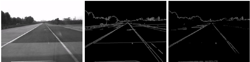
(a) The original image (b) The canny edge (c) The edge after double threshold
