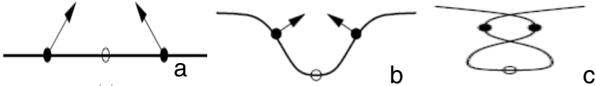
Fig. 3 Folding problem: (a) Displacing non-flipping vertices (dots) around solitary vertices (circle) may cause (b) folding of the mesh, and in an extreme case, (c) non-flipping self-intersection.
