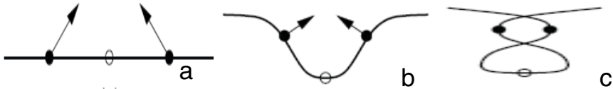
Fig. 3 Folding problem: (a) Displacing non-flipping vertices (dots) around solitary vertices (circle) may cause (b) folding of the mesh, and in an extreme case, (c) non-flipping self-intersection.
