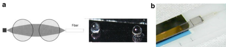
Fig. 22 (a) Picture of a micromachined Silicon micro-optical bench with ball lenses for optical coupling of an optical fibre with an integrate waveguide (end optics). (b) Magnified picture of a Pig-Tailing coupling of a Mach-Zehnder monolithic interferometer with an optical fibre (Front optics connection)
