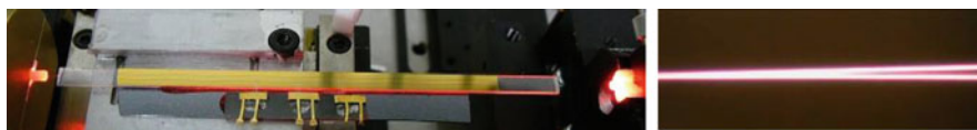
Fig. 21 Example of a complete Mach–Zehnder microinterferometer under test and a detail of one of the two Y-branches for fifty–fifty splitting/combining the radiation between the interferometric arms, which is one of the most critical points in the fabrication step
