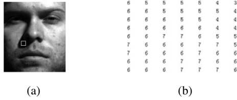
Fig. 1. Facial image. (a) facial image with white block (b) intensities of pixels in white block.
