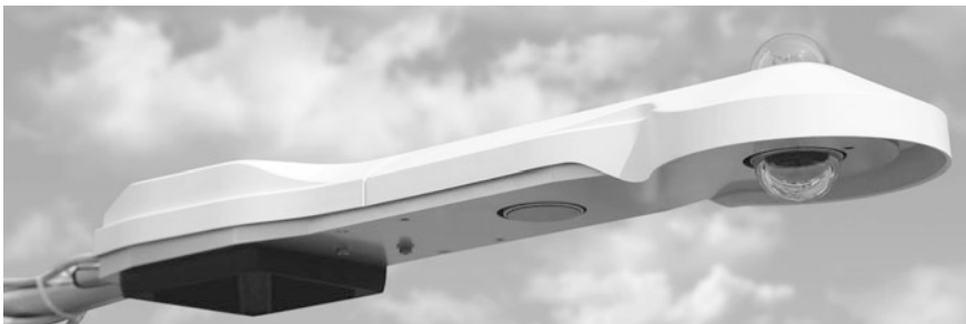
Fig. 6.7 Net radiometer CNR4 with two as albedometer installed pyranometer ( right ) and pyrgeometer ( middle ) and a common ventilation (published with kind permission of © Kipp & Zonen, All rights reserved)
