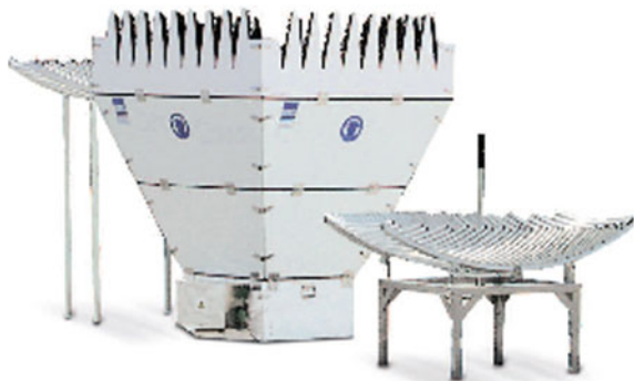
Fig. 6.20 Sodar-RASS system consisting on a “phased-array” Sodar ( middle ) and two radar antenna (published with kind permission of © METEK GmbH, Elmshorn, All rights reserved)
