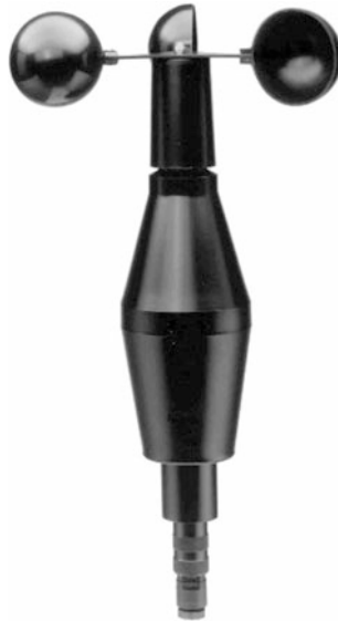
Fig. 6.8 Cup anemometer (published with kind permission of © Th. Friedrichs & Co., Schenefeld near Hamburg, All rights reserved)
