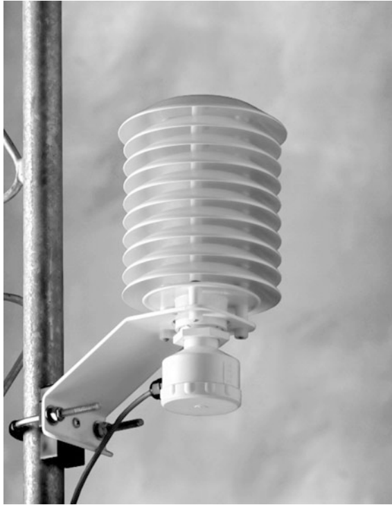
Fig. 6.17 Temperature hut according to Gill (model 41003) for micrometeorological investigations (published with kind permission of © R. M. YOUNG Company/GWU-Umwelttechnik GmbH, All rights reserved)
