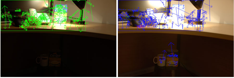
Fig. 1. An example of two aligned input images taken at different exposures. The arrows represent the scale, orientation and position of the SIFT features. The bounding box in each shows the areas within which SIFT features have been matched between the images using RANSAC during the alignment process [20].
