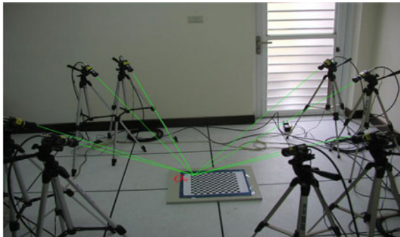
Fig. 3. Part of the multi-view video capturing configuration
