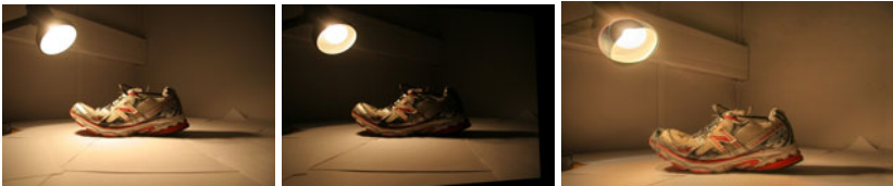
Fig. 6. A pair of stereo images at 10^\circ and a 2 EV difference, the second is warped to align with the first. The tone map image generated on the right hand side demonstrates the ghosting and other artefacts generated by tone mapping stereo images. Selecting SIFT features directly from the tone map can therefore generate unreliable features.
