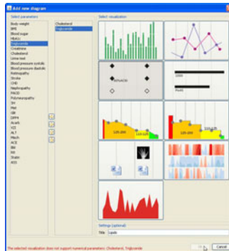
Fig. 2. Dialog to add a new diagram: Users select variables, a technique, and optionally a diagram title. The dialog will warn users, if they choose variables that are not supported by the selected technique. In the user study we used only bar chart, line plot, event chart, and timeline chart (top four options). The advanced visualization techniques were not visible in the user interface.
