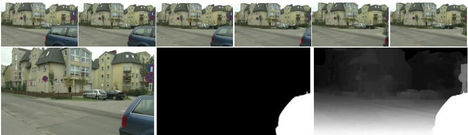
Fig. 11. The 427 th frame in the data set “Poznań”. (a) The reference frames. (b) The current frame. (c) The white region is the detected moving object. (d) Final depth map.
