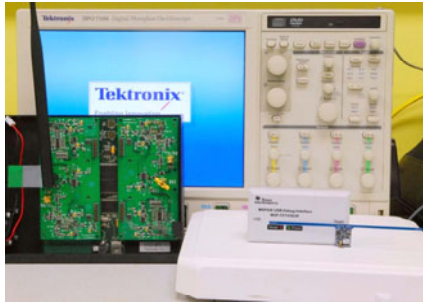
Fig. 6. Devices employed in our implementation and testing: one DP07104 oscilloscope, one USRP (v1.0), two RFX900 daughterboards, one VERT900 antenna, one circular polarity panel antenna, one WISP tag (v4.1) and one TI FET430UIF debugger
