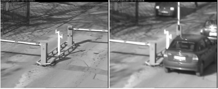
Fig. 4. Illustration of the focus loss problem. The defocused image (right) shows the lack of detailed information making it impossible to read the license plate.
