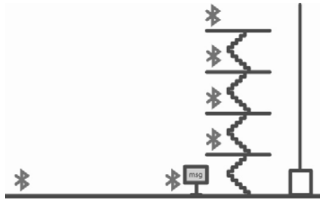
Fig. 1. Overview of the APStairs system: Users entering the office building are recognized by the first bluetooth scanner (left). Next, they are presented a message encouraging them to take the stairs. Finally, scanners in the stairway measure the success of the message.
