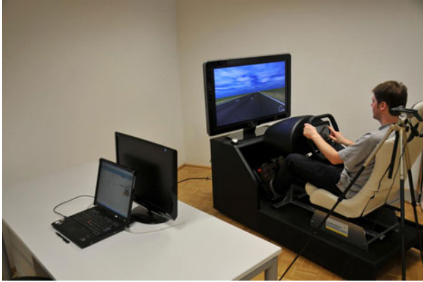
Fig. 2. LCT test setup with a fixed-base driving simulator
