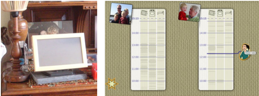
Fig. 1. A touch-screen display was used as an interactive awareness display in the homes of participating seniors and family caregivers (left figure). The display shows an activity trace for both the family caregiver and the senior in need of care (right figure). Users can add subjective annotations to the local activity trace, and can add question marks to the remote activity trace.
