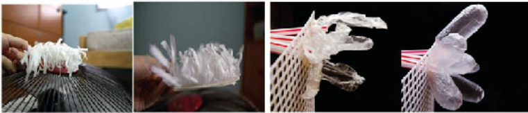
Fig. 1. (a) Initial position, (b) Strips raised 90* Fig. 2. (a) Deflated tubes, (b) Inflated tubes
