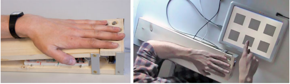
Fig. 1. The HapticArmrest (left) communicates tactile patterns and movements to the user's non-dominant hand. When touching an interactive element with the opposite hand, the user feels the form and surface characteristics of this item (right).
