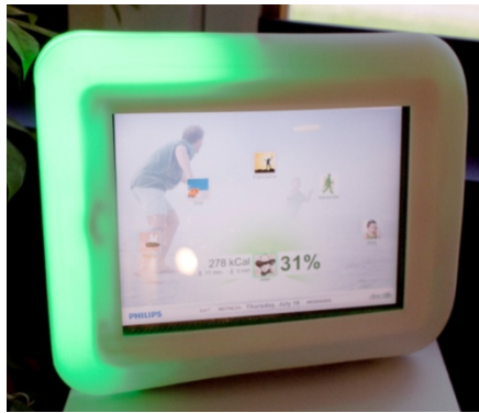
Fig. 2. Aulura’s interface with user activity level presented on both screen and frame. Clickable pictograms of friends and family are located around the user’s pictogram.
