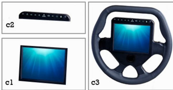
Fig. 1. Steering wheel design concepts: single touch (c1) multi-button (c2) and combi touch (c3)
