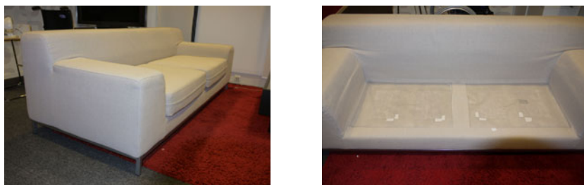
Fig. 3. An ordinary couch has been equipped with capacitive proximity sensors that have been set up under the upholstery and wooden elements
