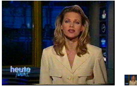
Fig. 1. Original image at 384 \times 288 and its DC image at 48 \times 36 . Frame extracted from the video I of the test set.
