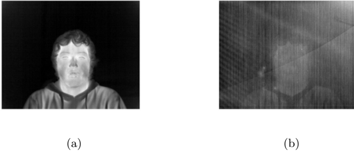
Fig. 1. Infrared images captured using the CEDIP JADE camera, a) free noise image and b) image with fixed pattern noise. The goal is to recognize the subject in an image as b).
