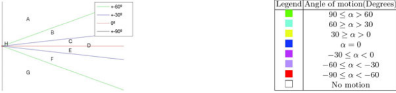
Fig. 4. Left: Diagram with the different types of possible direction in motion sequences. Right: Coding of the different directions of motion.
