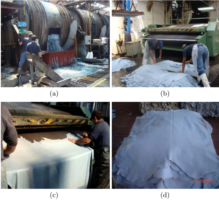
Fig. 1. Leather processing: (a) Ribera (b) Pre-classification (c) Drying (d) Wet Blue leather lot
