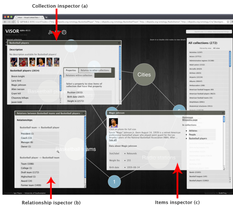
Fig. 3. Inspectors showing various information about the concepts in the ontology. Information about "Basketball Players" is shown in (a), and information about a particular basketball player (in this case Magic Johnson) is shown in (b). The various links that exist between "Basketball players" and "Basketball teams" is shown in (c).
