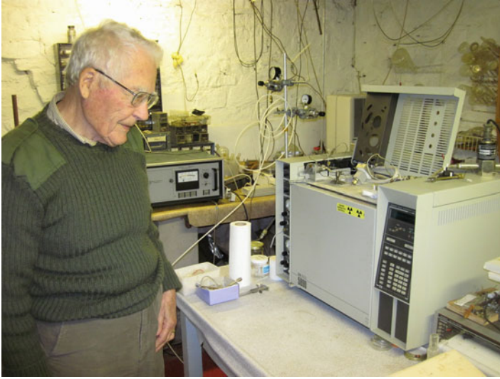
Fig. 2.6 James Lovelock (1919–) photographed in his lab in 2011 with a 1980s HP gas chromatograph – he was an advisor to Hewlett Packard on gas chromatography and used this technique in a number of groundbreaking studies of atmospheric chemistry studying an atmosphere in ‘extreme thermodynamic disequilibrium’ due to the presence of life. His concept of Gaia stresses the role of life as part of a single-coupled system, from which can emerge the sustained self-regulation of the Earth’s climate and chemistry at a habitable state for whatever is the current biota (Lovelock 2003. Photo: Dave Wilkinson)
