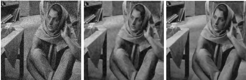
Fig. 5. Optimal correction experience. Left: Noisy image. Middle: NL-means solution. Right: NL-means corrected solution. The average with the noisy image makes the solution to be noisier, but details and fine structure are better preserved.
