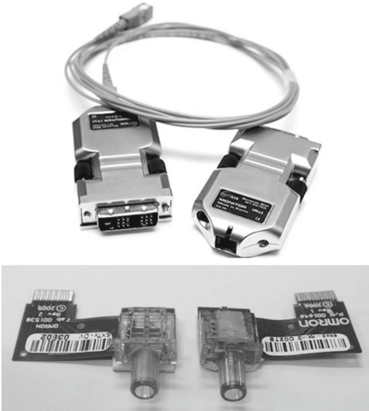
Fig. 15.18 Optical video link using internal CWDM optical sub-assembly
