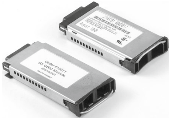
Fig. 14.12 GigaBit Interface Converter (GBIC) module, circa 1998. The GBIC was hot-pluggable, hot-swappable in the field giving customers greater flexibility and the ability to optimize configuration and deployment costs
