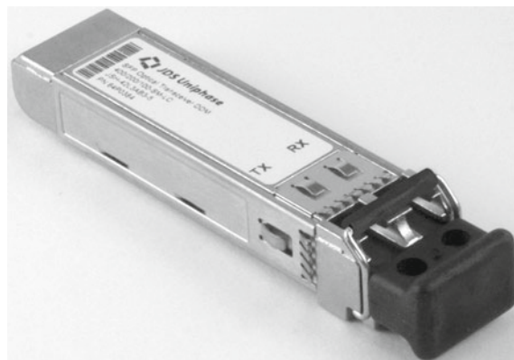
Fig. 14.10 Typical small form-factor pluggable (SFP) transceiver. The LC optical connector interface along with the high-speed serial electrical interface enabled higher density transceiver interconnects. The SFP transceiver is hot-pluggable and can be installed by the end-customer [7] (Courtesy of JDSU)
