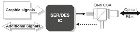
Fig. 15.20 One-fiber option using SER/DES and a bi-directional optical sub-assembly (OSA)
