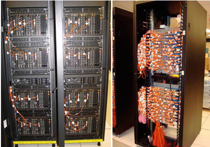
Fig. 16.31 Left: Front view of two compute racks from IBM’s Roadrunner system showing 4 Blade Center chassis each with 3 triblades and an active optical cable, right: rear view of an IB switch rack showing 2 switches and ~532 active optical cables
