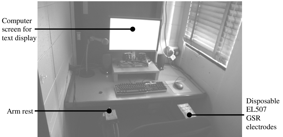
Fig. 2. The experiment was conducted in a room with a consistent environment for participants. A computer monitor displayed the reading text. The participants wore GSR equipment on their left hand, which they rested on the arm rest while reading.
