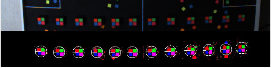
Fig. 7. Robot Traversal of a Spatially Varying Illumination Field. (Above) Consolidated Sequences of Robot's Motion, (Below) Robot Tracking Results. White circle denotes the recognised robot and the white line segment denotes the calculated robot heading angle.
