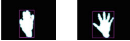
Fig. 4. The result after skin detection, showing human hand with two states, in the left is the human hand with the fingers are together, and in the right when the fingers are apart
