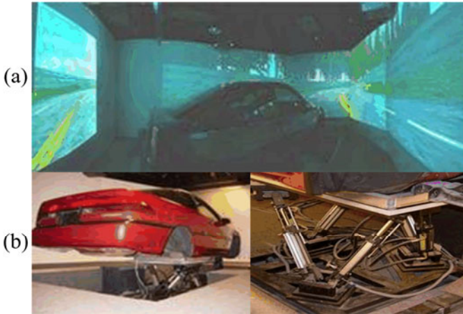
Fig. 1. VR-based Highway Driving Environment. (a) Snapshot of the virtual reality-based driving scene, (b) six degree-of-freedom motion platform.
