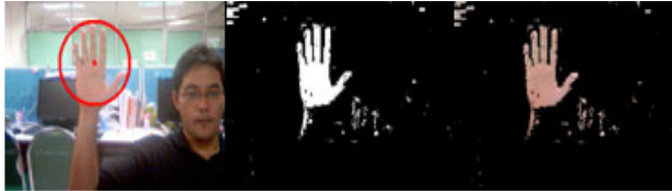
Fig. 5. Hand tracking with CamShift
