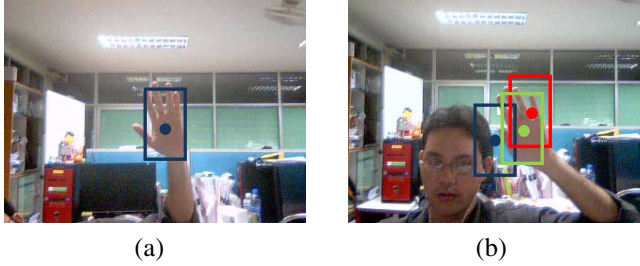
Fig. 7. Kalman filter (a) Position from CamShift for prediction in the next frame (b) Estimate new hand position (green dot) between CamShift (blue dot) and prediction (red dot)
