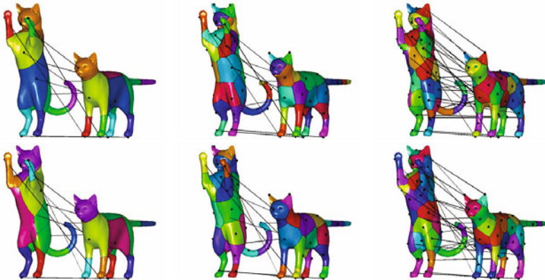
(d) The Laplace-Beltrami operator-based descriptors and geodesic distance metric; the upper row - same orientation correspondence, the lower row - the reflected one.
