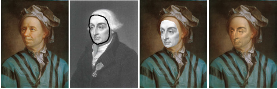
Fig. 3. Seamless image cloning with osmosis (with permission from [19]). From left to right: (a) Original painting of Euler. (b) Original drawing of Lagrange (with to-be-cloned face selected). (c) Direct cloning on top of Euler’s head. (d) Cloning with osmosis image editing. See [19] for more details.
