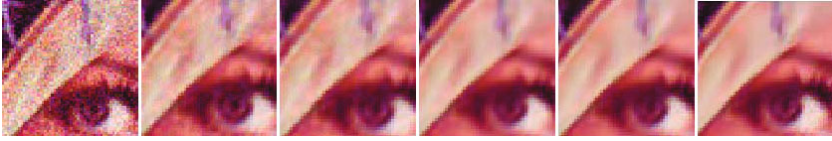
Fig. 5. Optimized denoising for different values of K a) Noisy image, \sigma = 20 , PSNR = 22.25 b) PSNR = 28.93 , K = 1 c) PSNR = 29.91 , K = 2 d) PSNR = 31.15 , K = 5 e) PSNR = 31.45 , K = 10 f) PSNR = 31.55 , K = 40
