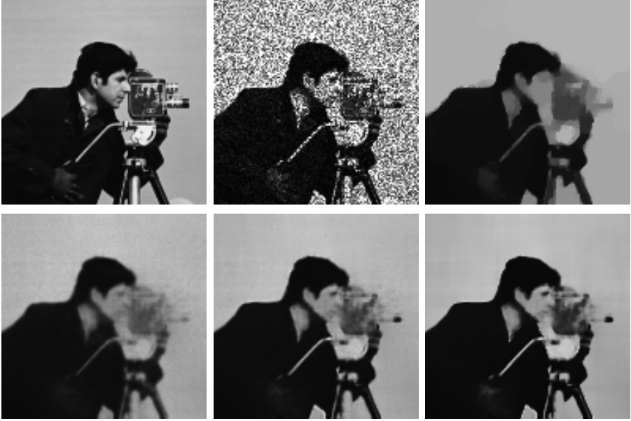
Fig. 5. Top: Original image with values in [0, 255] (left), corrupted version by multiplicative Gamma noise with L = 4 (middle) and restored image by the I-divergence - TV model as presented in [14]. Bottom: Results by our new nonlocal filter (6) using just (17) with l = 7 , \omega = 29 , a = 1.5 , h = 1 (left), using (18) with q = 0.35 (middle) and after an additional updating step with \tilde{l} = 3 , \tilde{a} = 0.5 , d = 0.25 (right).
