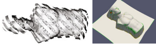
Fig. 6. On the left \mathcal{G}_{r_0} for time averaged real ToF data and the underlying CT phantom \mathcal{G}_{CT} are rendered in a single image using alternating slices. On the right the distance \text{dist}(\phi(\mathcal{G}_{r^*}), \mathcal{G}_{CT}) on \phi(\mathcal{G}_{r^*}) is again color-coded as in Fig. 2
