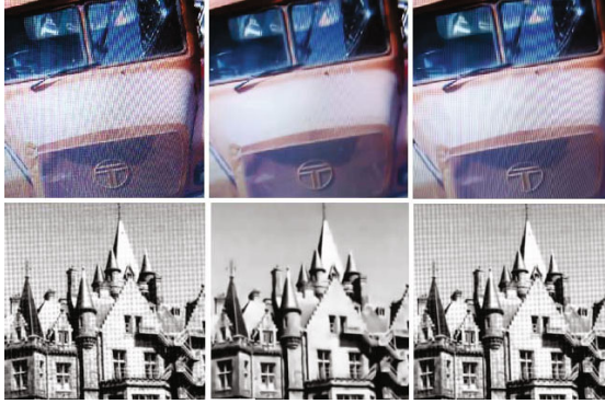
Fig. 7. Removal of aliasing and block textures. From left to right, top to bottom a) Photograph of truck with aliasing. b) Beltrami patch denoising, \sigma = 20 c) CBM3D denoising, \sigma = 20 d) Photograph of castle with weak block textures e) Beltrami patch denoising, \sigma = 20 f) BM3D denoising, \sigma = 20 .
