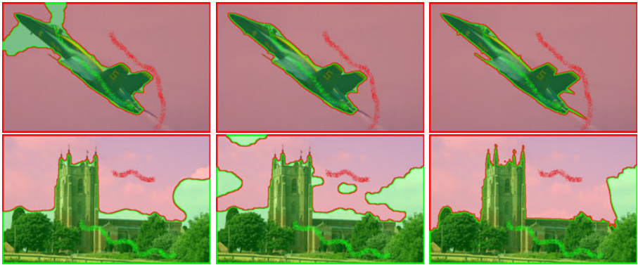
Fig. 4. Comparing different regularization terms in terms of interactive multi-label segmentation ( cf. [27]): TV regularization (first column), edge-weighted TV regularization (second column) and the proposed non-local variant (third column). The scribbles are the users input to mark the corresponding region.
