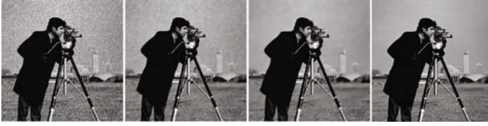
Fig. 4. From left to right a) Noisy image at \sigma = 20 b) Denoised with 10 iterations, PSNR = 29.21 c) Denoised with 150 iterations PSNR = 29.35 d) Original image
