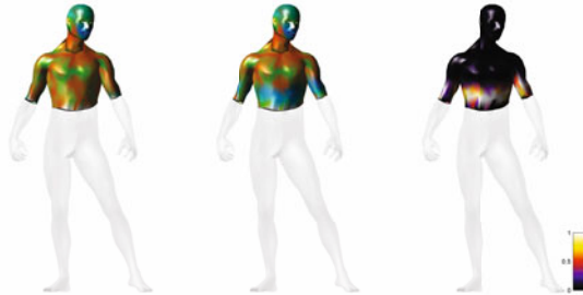
Fig. 1. An RGB visualization of the first three component of HKS descriptors computed on the full shape (left) and on a part of the shape (center). The L_2 difference between the two fields is depicted in the rightmost figure. Note that the difference is maximal on the boundary decaying fast away from it; the error decay speed depends on the scale choice in the HKS descriptor.
