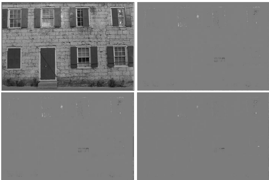
Fig. 4. Top-left corner: the given true quantized image w . The difference image between w and the output image v by LM method (top-right), WA method (bottom-left) and our method (bottom-right). Our method yields fewest features in the difference images.
