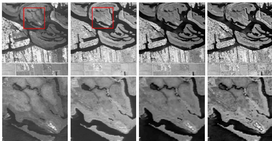
Fig. 4. Fusing images from two spectral bands. At 1st row: the left two images show the input images of remote sensing images from two different spectral channels; the right two images show the fused images computed by (1) and (3) respectively. At 2nd row: the left two images show the zoomed image patches cropped by the red lines on the same position of the input images respectively; the right two images show the fused results at the patched area computed by (1) and (3) respectively.
