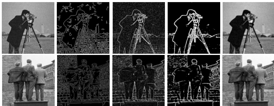
Fig. 3. Column 1: original images; Column 2: detected edges by the Canny method; Column 3: detected edges by the Ambrosio-Tortorelli method; Column 4: detected edges by our proposed method; Column 5: reconstructed image u by our proposed method.
