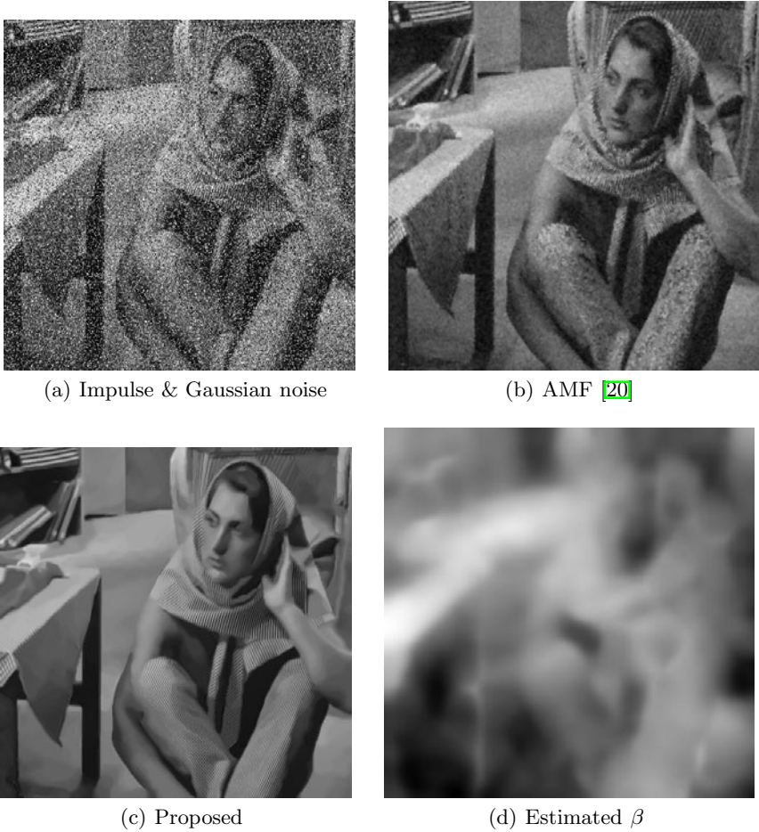
Fig. 2. Results under impulse noise plus Gaussian noise. (a)noisy image; (b) denoising with adaptive median filter (AMF) in [20], PSNR=23.47; (c) denoising with the proposed model, PSNR= 27.16 ; (d) the estimated bias function \beta ;
