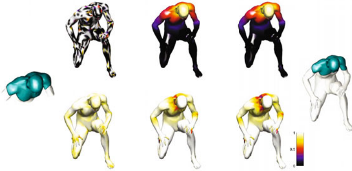
Fig. 2. Convergence of the alternating minimization procedure. Depicted are the membership function \mathbf{u} (top row) and the phase field \rho (bottom row) at the first three iterations.
