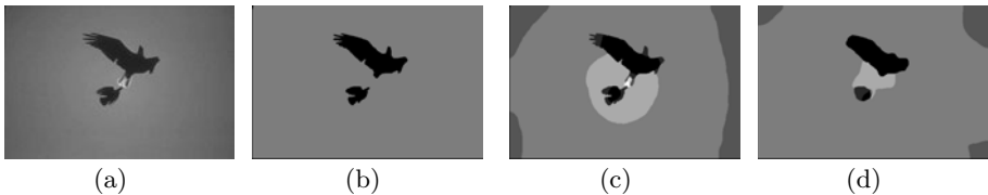
Fig. 1. (a) shows the given image. (b) shows the image partition result of (3) computed by the proposed method in this paper. It gives only two segments left along with properly smoothed boundaries! (c)-(d) show the partition results computed by the Potts model (5) without the label cost prior, which give the results either oversegmented (more labels) or oversmoothed. In this example we have used 11 evenly spaced labels.
