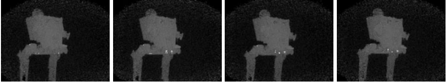
Fig. 4. Four exemplarily selected frames of a sequence of depth maps taken with a time-of-flight camera
