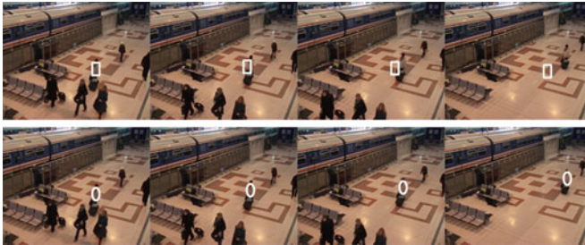
Fig. 4. Tracking results in the passenger sequence with the traditional covariance tracking method (top) and our proposed one (bottom)
