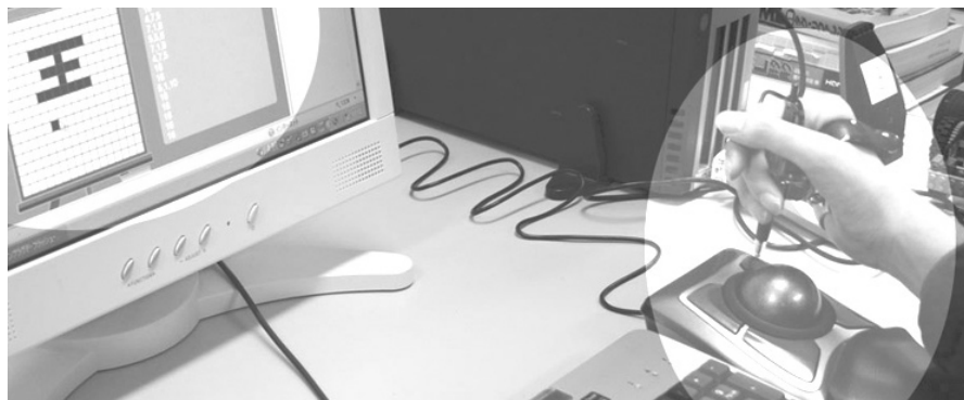
Fig. 3. Student with impairment using upper clicked trackball with special equipment for drawing/painting
