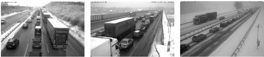
Fig. 4. Examples of the display of automatic switched alarm images for the Level of Service “traffic congestion” under different conditions. Left image: occlusion in driving direction, middle image: occlusion sideways, right image: fog and snow.
