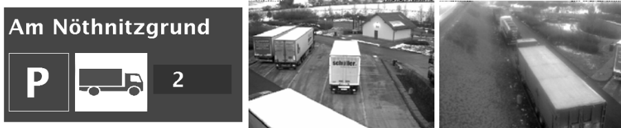
Fig. 8. Programmed information board with the amount of free parking spaces. The result can be verified by the image in real-time. The right image shows an example for triggering an alarm image while someone was parking in the exit of the parking area.
