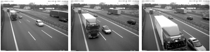
Fig. 1. Example of the rapid change of vehicle size in an image sequence with a camera high of 7.5 m. As a consequence, the tracking of the object across the whole image is difficult to accomplish.
