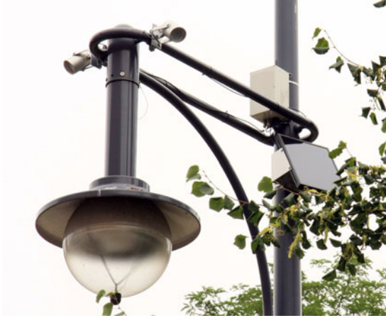
Fig. 4. Prototype of the modular traffic monitoring module (mounted on a lamp pole, with solar panel and two Passive Infrared Detectors for adjacent lanes) [5]
