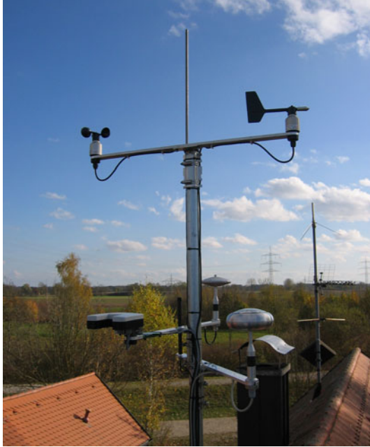
Fig. 2. Completely equipped sensor station with developed wind and precipitation sensors (bottom right) in combination with reference sensors (bottom left and top)
