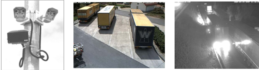
Fig. 6. Typical view of a camera installation with infrared light on a 10 m pylon. The right image shows a typical situation at the exit of the parking area at night.
