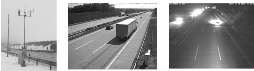
Fig. 2. A typical camera installation with example images for day and night. The lights on the vehicles in the right image are sufficient for our image processing algorithm. The camera uses the power supply of a meteorological station.
