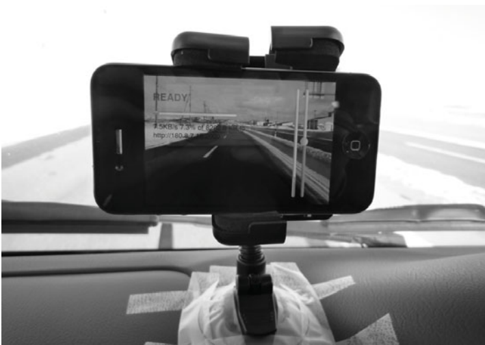
Fig. 3. Scene from driving experiment showing smart device image, acceleration and GPS data collection display, and real-time transmission
