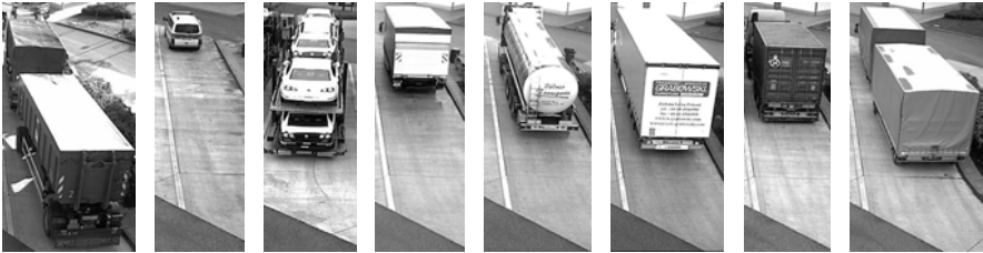
Fig. 5. The use of non-specific vehicle features is necessary to consider different types and sizes of vehicles. Small vehicles can be anywhere on the parking space, so an analysis of the whole area is necessary.
