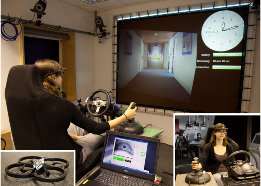
Fig. 3. The driving simulator, adapted for remote control of the Parrot AR.Drone
