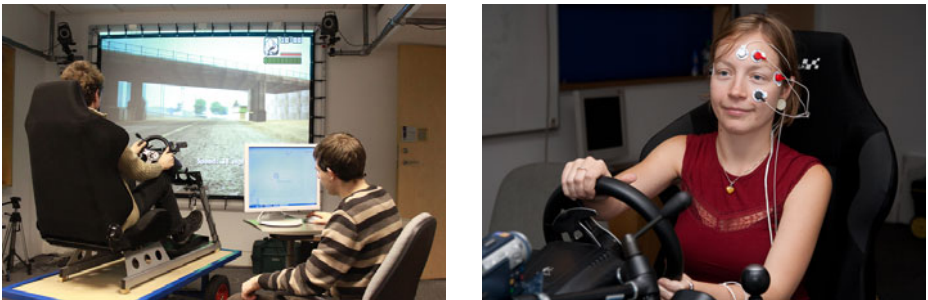
Fig. 1. Participants were asked to drive through several scenarios in our fixed-base driving simulator while wearing EOG, GSR and BVP physiological sensors
