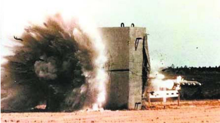
Fig. 12.2 A test for penetration and perforation of concrete slab (Sandia crash test)
