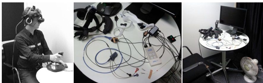
Fig. 2. (left) An example of the complete setup; (middle) The experiment room with HMD, joystick, physiological sensors, fan, and desktop monitor; (right) The "VarioPort" biometrical device with sensors for skin conductance, ECG, finger pulse, and chest measurement, plus remote marker buttons
