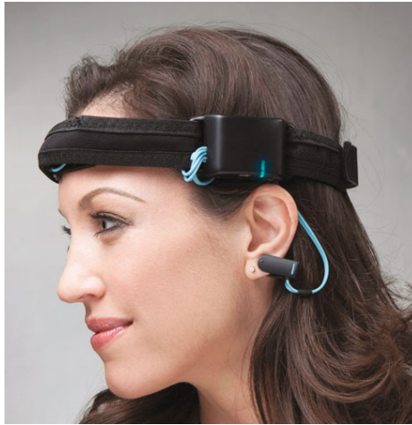
Fig. 1. Two-channel dry-sensor EEG device. The EEG device is housed in a headband form factor with two dry sensors placed at the inner side of the headband on the forehead (FP1 and FP2). The EEG circuitry is located inside the black case at the left side of the head. A power switch at the bottom of the case serves to turn on/off the device. A mini-USB port, also at the bottom of the case, is for charging a lithium-ion battery that provides power to the device. A blue light outside the case will start to flash when the device is turned on; and it stays on continuously when the device is communicating to a computer via Bluetooth connection. An on-board 8MB flash memory inside the case can store up to 3.5 hours of EEG data.
