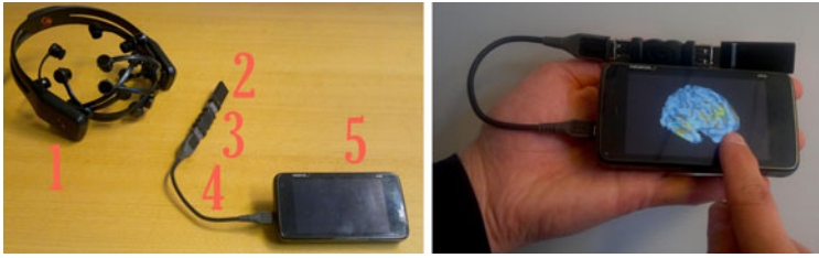
Fig. 1. (left) The system with Emotiv EPOC wireless EEG headset (1), Receiver module with USB connector (2), USB connector and adapter (3+4), and Nokia N900 (5). (right) Touch-based interaction with a 3D model of the brain using the smartphone.
