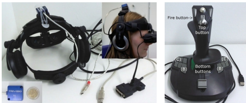
Fig. 1. (left) TriVisio's "VRVision" HMD with the "Colibri" tracker (down left) attached; (right) The "Thrustmaster T-16000M" joystick for navigating the virtual emergency scenario
