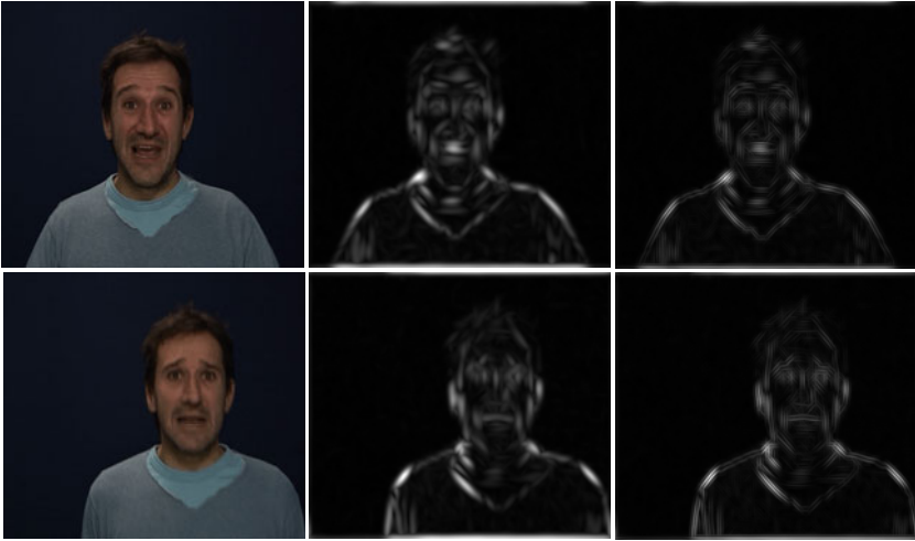
Fig. 1. Left column: facial images with a given emotion. Middle : Energy filter output. Right : Standard Gabor filter output.
