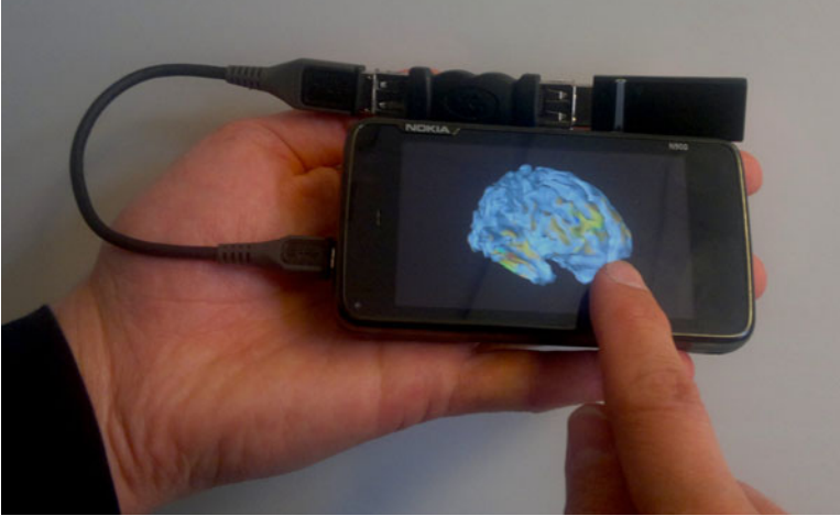
Fig. 1. The wireless neuroheadset transmits the brain imaging data via a receiver USB dongle connected directly to a Nokia N900 smartphone. Reconstructing the underlying sources realtime from the EEG data in a sparse 3D model improves decoding of the signal and potentially provides relevant neurofeedback for brain machine interfaces.
