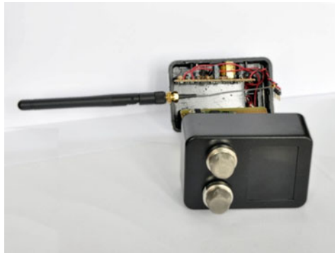
Fig. 3. A snapshot of one of the ZigBee-equipped smart sensor node used for our experiments. The whole device is based on low-cost components.
